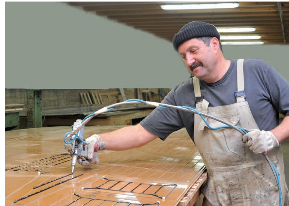
Verfugung der CNC gefrästen WOLZYNTEEK-Paneele. Joining of CNC-milled WOLZYNTEEK panels.
